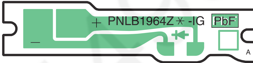
KX-TG7841/7842/7843/7844/7845/365/7871/7872/7873/7874/7875/385 CIRCUIT BOARD (Base Unit_LED (Component View))
