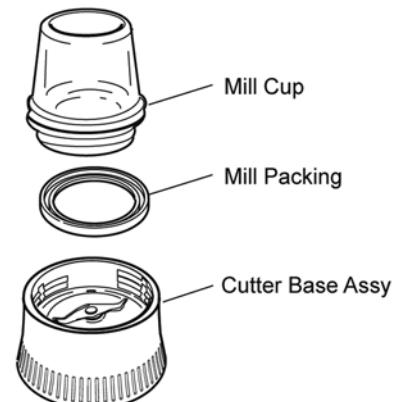
2. The safety device lever from the cutter base assy can be removed after its three screws are loosened. (Make not lose a spring).
