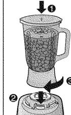
Place ingredients into blender container. Ensure the cover is firmly in place to avoid ingredients flying out. Place container on motor housing. Twist container clockwise to lock.
