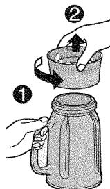
Turn blender container base counter-clockwise to disassemble.
