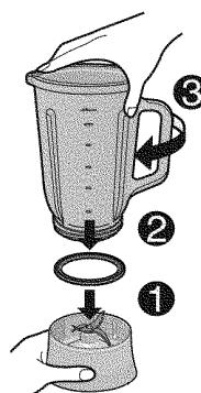
Turn blender container clockwise to assemble.
