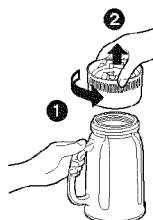
Turn blender container base counter-clockwise to disassemble.
