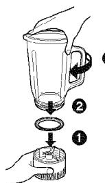
Turn blender container clockwise to assemble.
