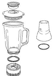
Wash the parts using a soft sponge soaked in diluted kitchen detergent (neutral). To remove ingredients stuck in the cutter, carefully clean it with a brush. Then rinse thoroughly with water, and allow the parts to dry out.
