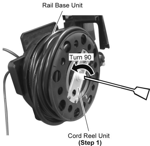
**Step 2** Remove Cord Reel Unit from Rail Base Unit.
