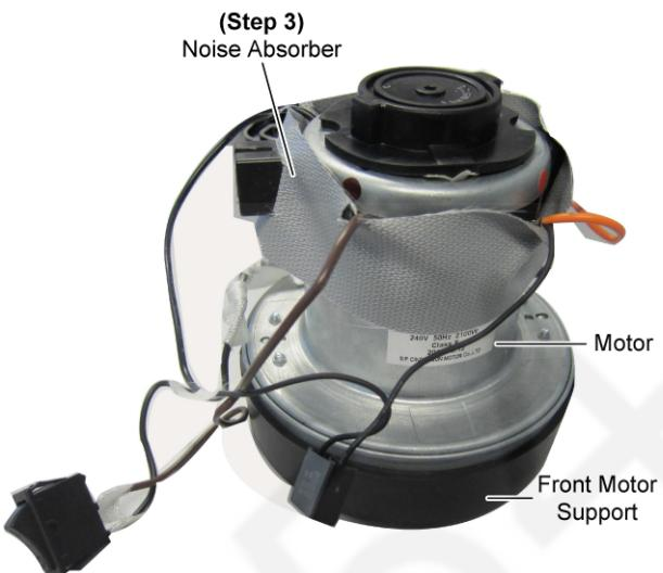
**Step 2** Release Wire Connectors from Motor.
