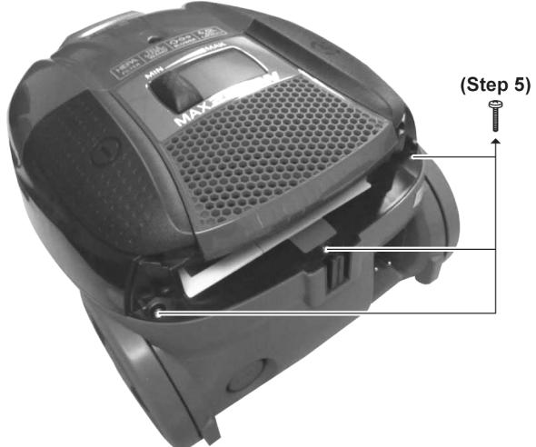
**Step 6** Hold the Upper Body and 1 of the wheel to lift up the Upper Body.
