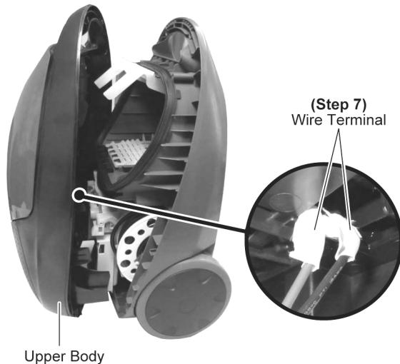
**Step 8** Remove the Upper Body from Lower Body.
