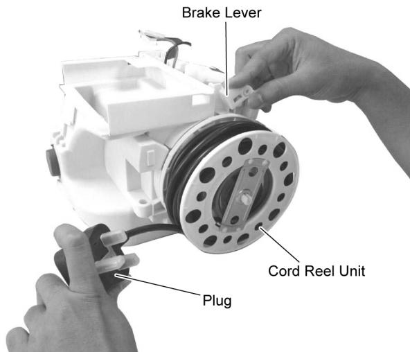
**Step 2** Remove the Cord Reel Unit from the Motor Case Set by inserting a slotted screwdriver into the shaft of the Cord Reel Unit and turning it 90° counter-clockwise.
