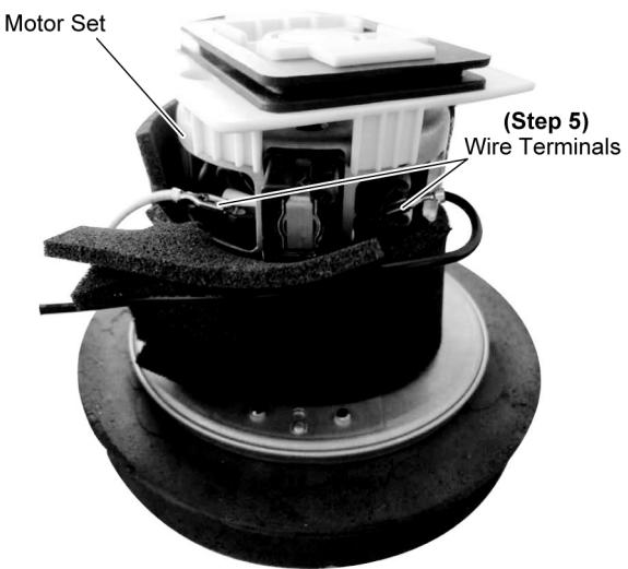
**Step 6** Remove the Noise Supprassor Unit and Motor Support Rubbers.
