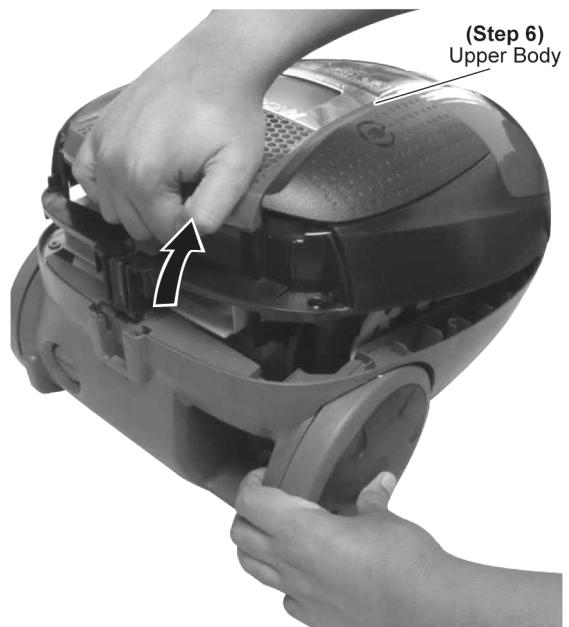
**Step 7** Place the set as diagram shown and disconnect the Wire Terminal from switch at the Upper Body.
