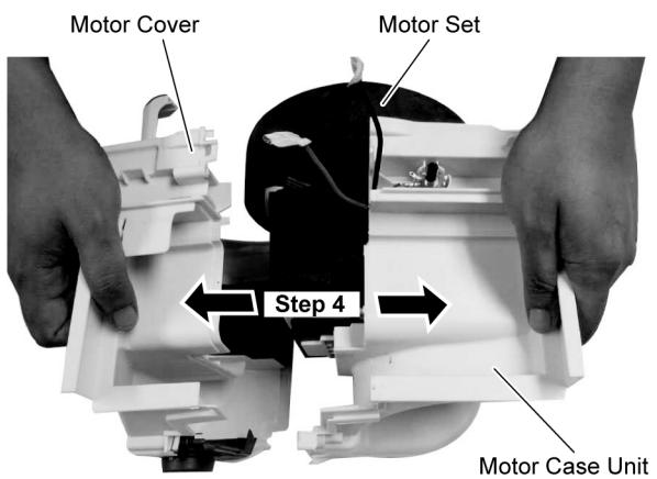
**Step 5** Disconnect the Wire Terminal and remove the Motor Set.
