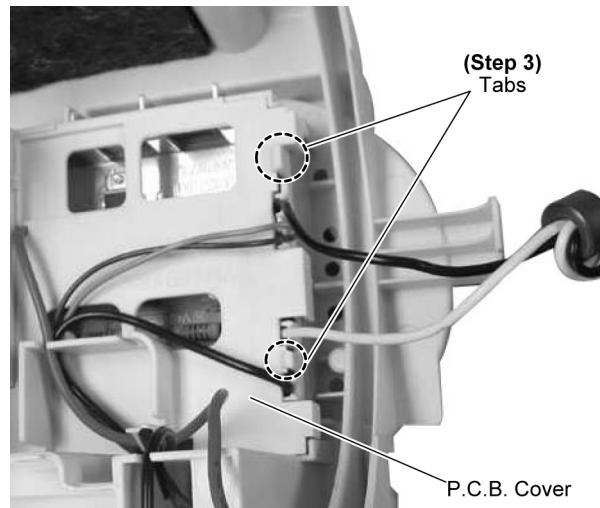
To reassemble the unit, reverse the disassembly procedure above.
