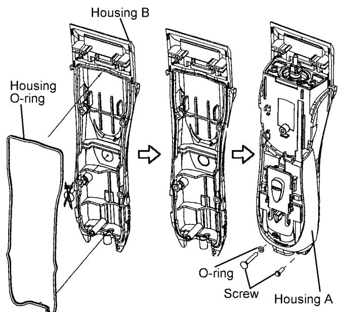
5. Set the trimmer. And tighten four housing screws.
