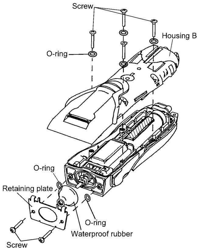
13. To take out the motor assembly, lift up the lead wire side of motor and pull it towards the battery side in the direction of arrow.
