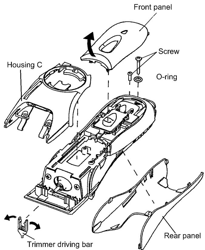
9. Loosen four screws with O-rings.
