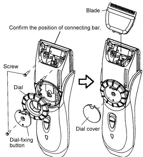
After assembling the unit, confirm the smooth up and down operation for attachment. And confirm if the dial shows "20" when the attachment is the highest position.
