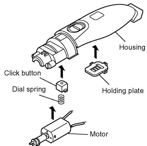
2. Place the holding plate on the housing A firmly.
