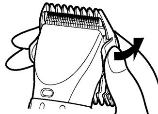
2. First, hold the handle of the hair clipper firmly with the "Panasonic" name facing upward and set the dial to "2.0mm", and push the upper part of the blade away from the housing.
