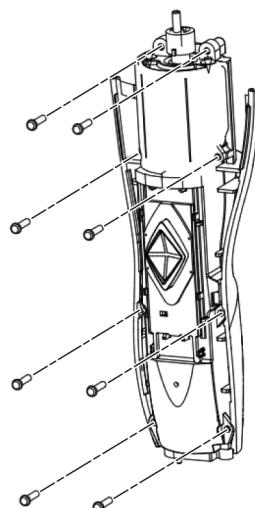
7. Separate the housing B from the housing A.
