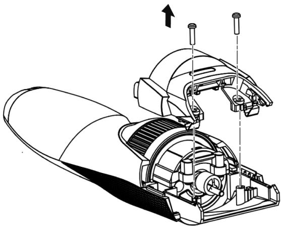
3. Loosen a screw from bottom cover.
