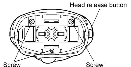
2. Open the housings with pushing the head release buttons.
