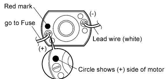
2. Press fit the lead wires into housing neatly.
