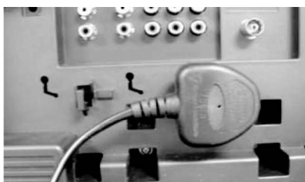
Fix AC cord at back cover 3 pin plug
