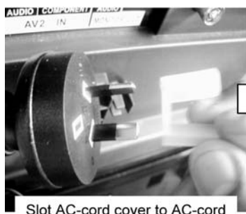
Slot AC-cord cover to AC-cord
