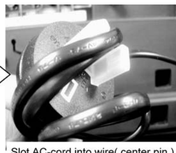
Slot AC-cord into wire( center pin )
