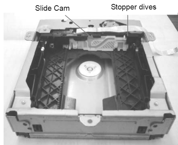
After fall down of Traverse Base
