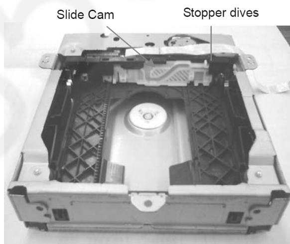
After fall down of Traverse Base
