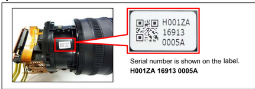
Fig-1. Location of the Camera Lens Unit Serial Number
